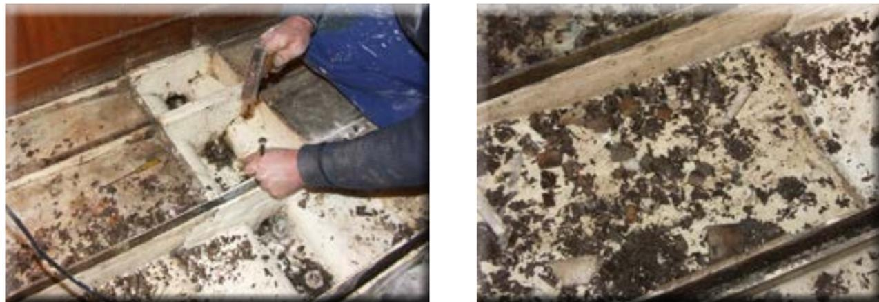
Mouldy wood can be easily removed from the laminate with a pointed object (peat cutting)
