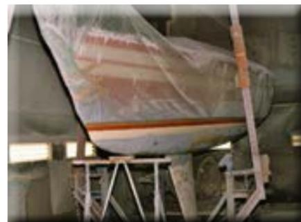
Hull is masked off for further work steps after drying
