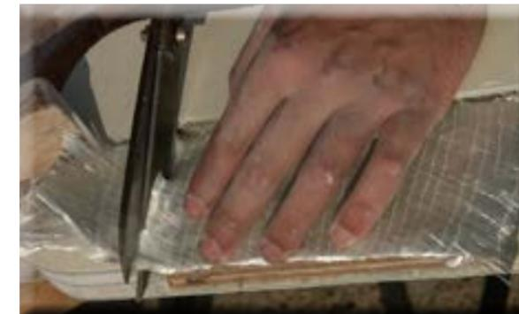
Cutting the reinforcing fibers
