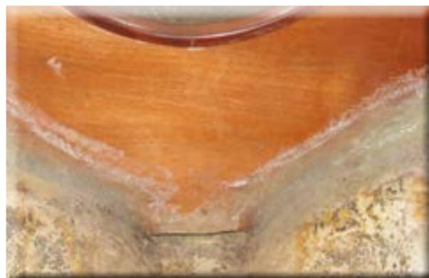
Crack in transition main bulkhead to bilge
