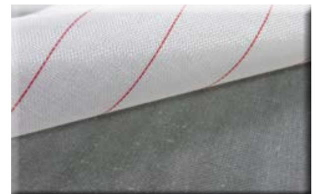
Surface after tearing off the fabric
