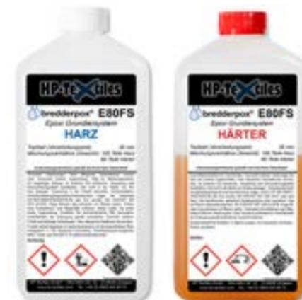
As soon as the surface has gelled, the subsequent layer of epoxy resin can be applied. If the subsequent layer is not applied within 24 hours at 20°C, it is mandatory to sand the entire surface. Substrates unsuitable for bonding or laminating are, for example, PE, PP, soft PVC, PTFE and some other special plastics. In case of doubt, we recommend preliminary tests.
