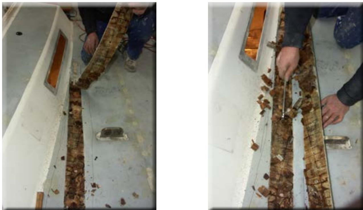
Yielding decking suggests damage to the laminate and this extent becomes after opening recognizable
