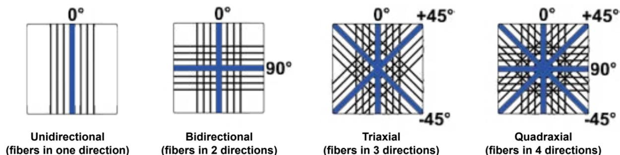
**Glass filament fabrics** are webs of continuous E-glass produced by a weaving process. The basic mechanical properties (tensile strength, tensile elongation, E-modulus and elongation at break) are determined by the type of glass, the application properties, but above all by the sizing and the type of weave.
